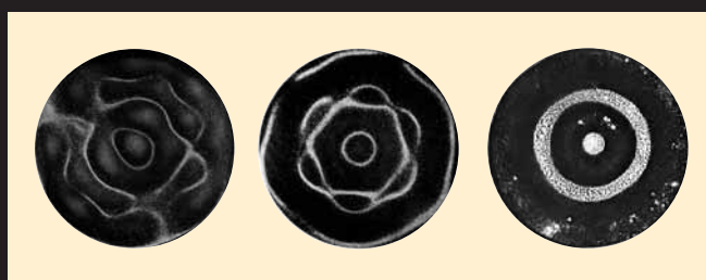
Top: Fig. 2 Ernst F.F. Chladni demonstrates 'nodal patterns' by bowing a small steel plate covered with sand. Bottom: Fig. 3 Sound figures formed on a rubber membrane. Left to right: 'oh', 'ah', and 'oo'. 5 ©2001 MACROmedia Publishing.
